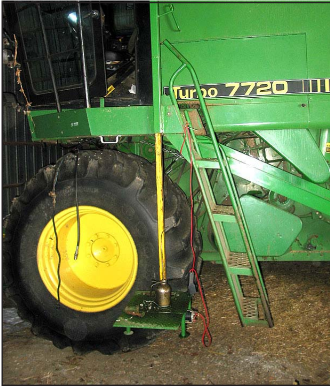
Figure 1. Platform lift on the combine.
