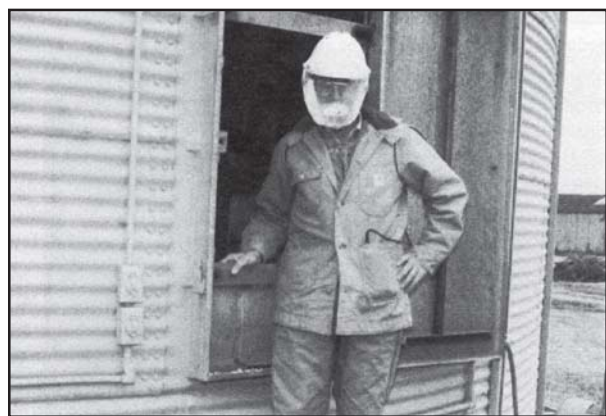
Figure 8. The air stream helmet forces filtered air over the face of the user. The moving air makes breathing easier and the user cooler.
