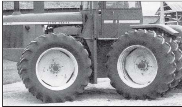
Figure 11. Articulated-steered tractors present another kind of hazard. Should this man-lift be in the down position when the tractor is turned, it would be crushed between the front and rear tires.
